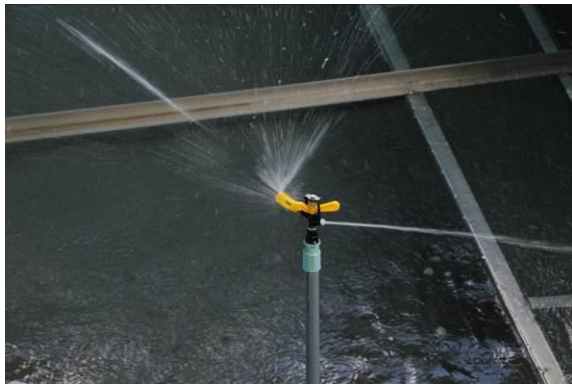
Water spray to clean the wall
