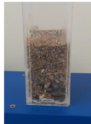
Figure 11 Filter Tank (4 basins) and arrangement of materials in the filtration unit
